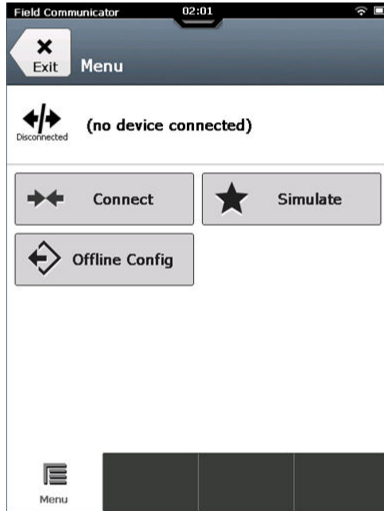
Figure 3-7: Menu screen for no connected HART device
