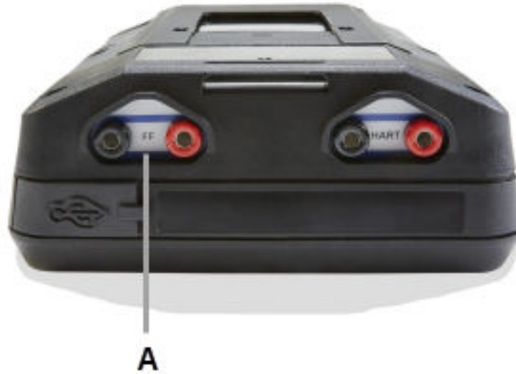
Figure 3-37: FOUNDATION fieldbus terminals on the Device Communicator communication module
