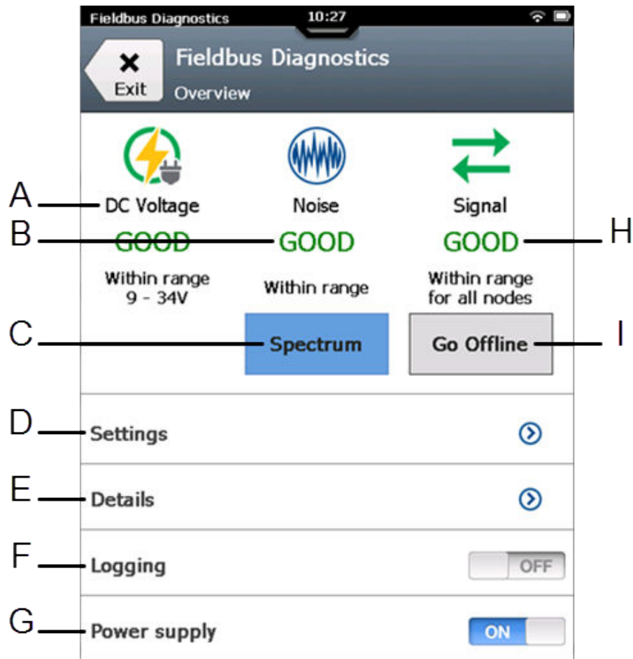
Figure 5-2: Fieldbus Diagnostics Overview screen while taking measurements
