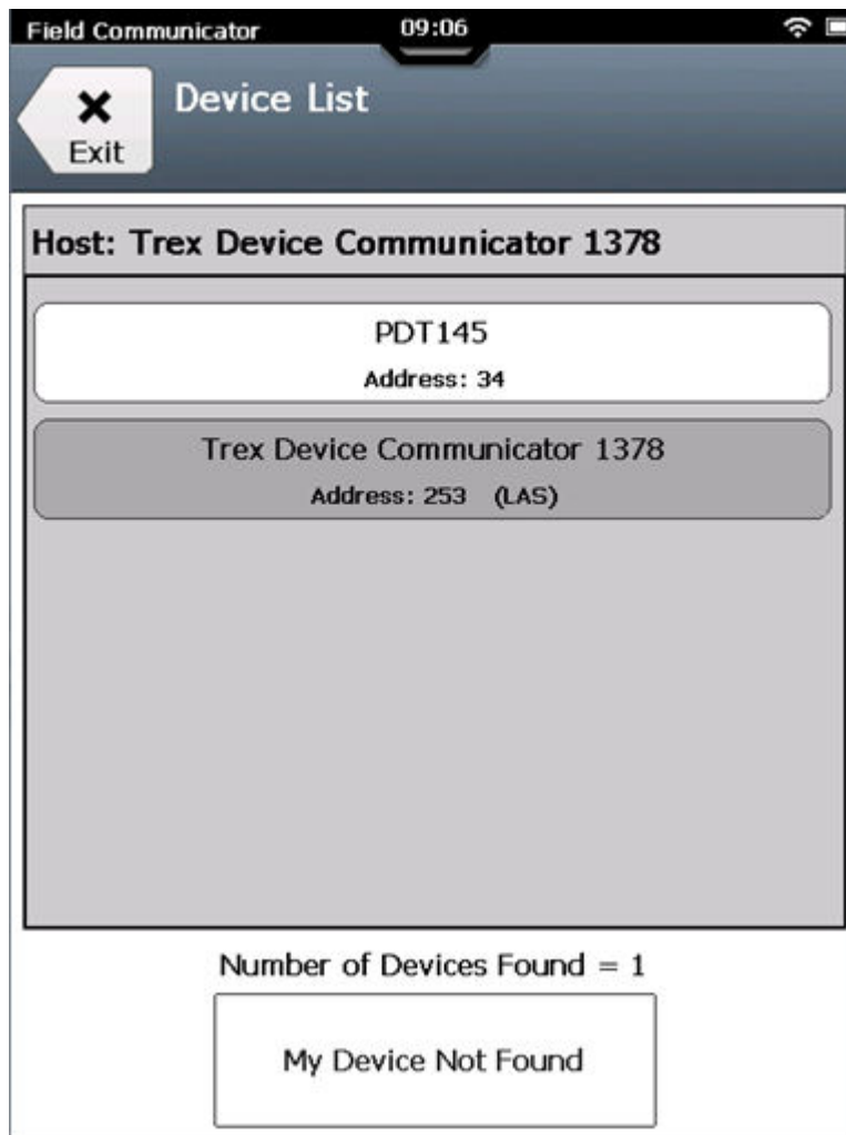
Figure 3-41: Fieldbus Device List
