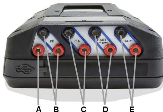
Figure 2-5: Device Communicator Plus communication module
