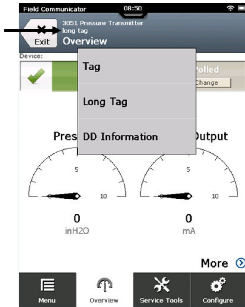
Figure 3-45: Tap the device tag
