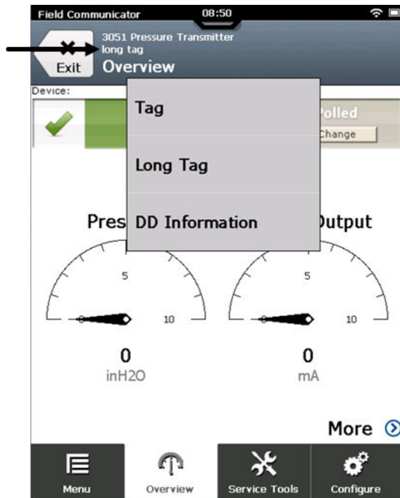
Figure 3-33: Tap the device tag
