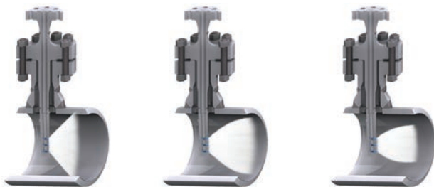
Figure 3: Attemperator overspray, proper spray, and underspray.
