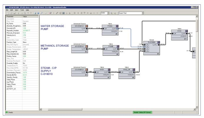
Unit operation objects are used to quickly develop accurate models for testing and training.
