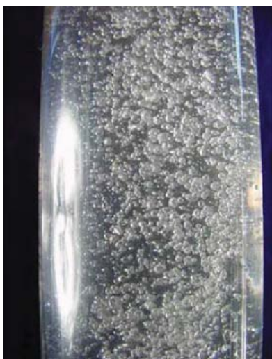
Figure 7. Entrained gas bubbles
