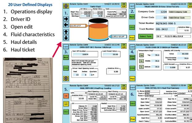
Figure 7: Well pad tank management haul interface
