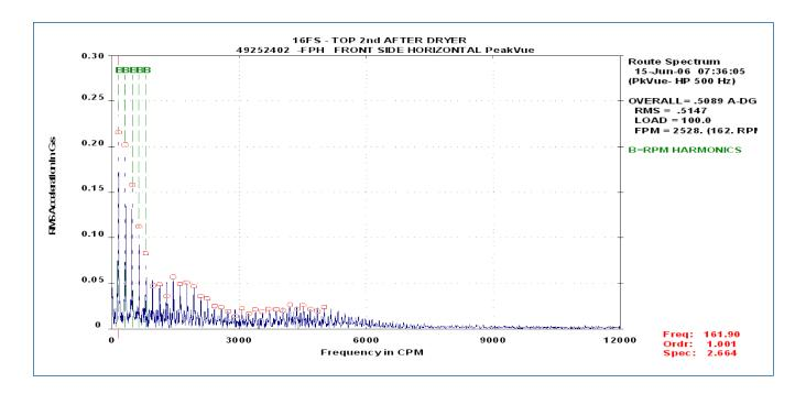
Three PeakVue readings were collected at that time, which are displayed in the waterfall plot below. The middle June 15th reading was taken when the audible noise decreased. An analysis of the collected data was performed and a report generated. Recommendations were made to increase monitoring of the bearing PeakVue and temperature values until maintenance could be performed. An inspection of the bearing for looseness or wear was also recommended at the next opportunity.
