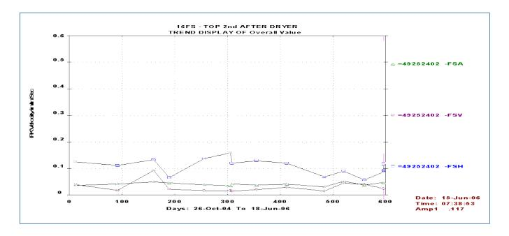
PeakVue data contained multiples of TS, and the overall PeakVue value increased when the audible noise was louder.
