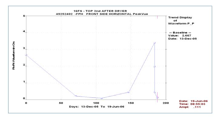
A TM shutdown was scheduled for June 20th and an inspection of the After-dryer T2 Roll bearing was performed at that time. The inner race was found to be loose on the shaft. Measurements on the journal found it to be severely worn where the bearing inner race was spinning on the shaft. A compression fit is used on this configuration to hold the inner race in-place on the roll journal. The journal was machined and a sleeve was installed along with a new bearing.
