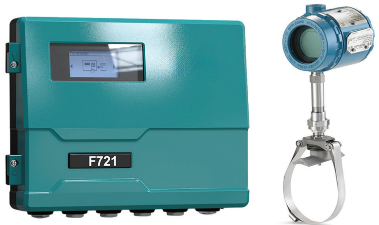
FIG. 7. Non-intrusive, clamp-on ultrasonic flowmeter e (left) can measure flow through a heat exchanger without a process penetration. Similarly, X-well temperature transmitters (right) can measure temperature through the pipe wall, so these instruments can be added without process shutdowns.
