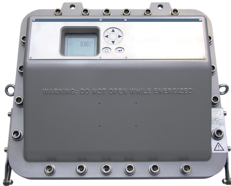
FIG. 5. Gas analyzers, like the proprietary technology c shown here, use non-dispersive infrared photometric detectors to detect and quantify components common to SMR, helping guide operators as they monitor the effectiveness of each subsequent step.
