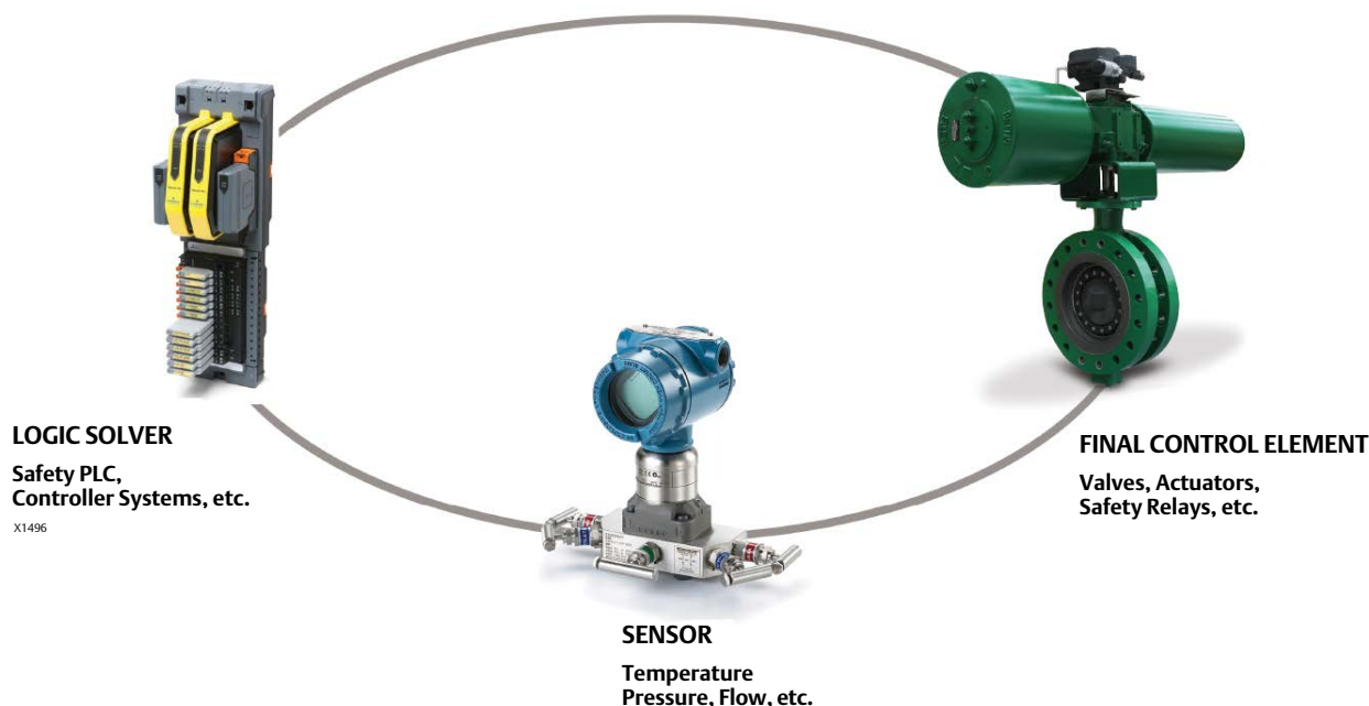
Figure 2. Components of a Safety Instrumented System
