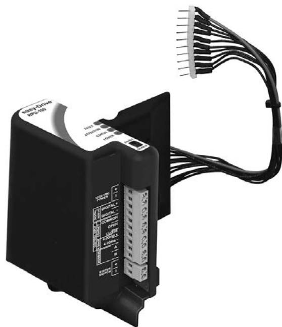
Figure 1. Fisher RPU-100 with Wiring Harness
