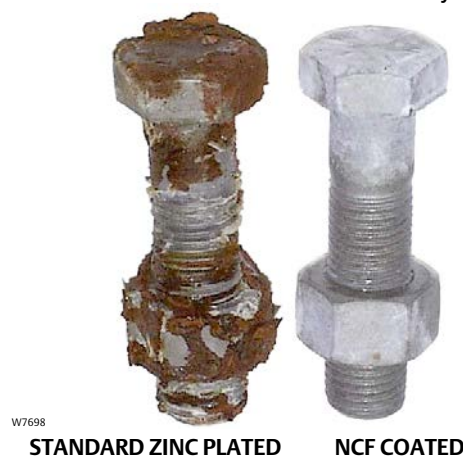
Figure 6. NCF-Coated Fasteners Exhibit Superior Performance in Accelerated Laboratory Tests
