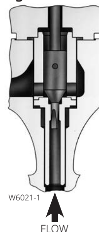
Figure 18. Fisher HPT Trim with Whisper Trim III Level A1 Cage (also available in HPD NPS 2 to 6 and HPS NPS 2 and 3)
