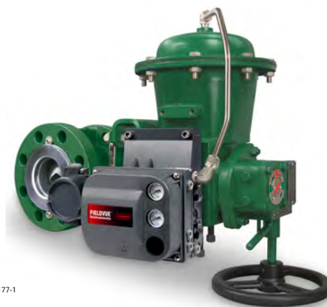
FISHER 1078 DECLUTCHABLE MANUAL ACTUATOR MOUNTED ON A 2052 SIZE 1 ACTUATOR AND V300 VALVE WITH FIELDVUE™ DVC6200 DIGITAL VALVE CONTROLLER
