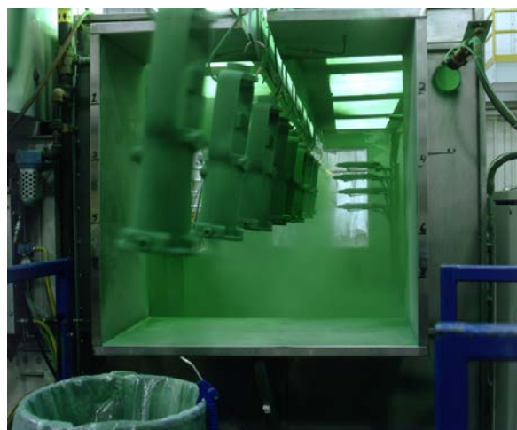
Figure 3. Powder Coating is Nearly 100% Free of VOCs
