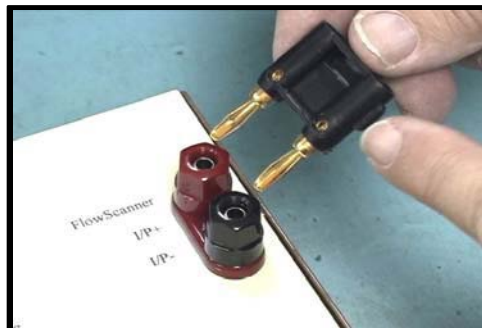
Figure 4. The tab on banana plug indicates the negative side
