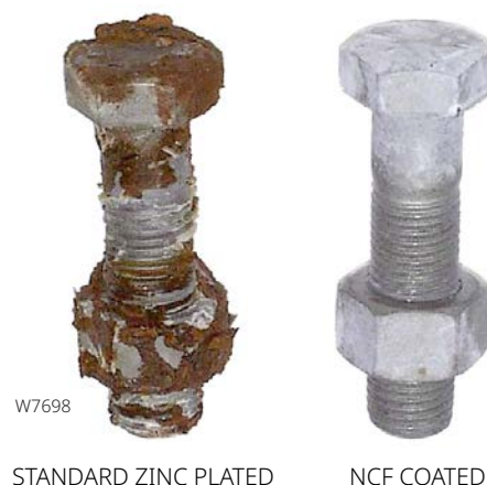
Figure 5. NCF-Coated Fasteners Exhibit Superior Performance in Accelerated Laboratory Tests
