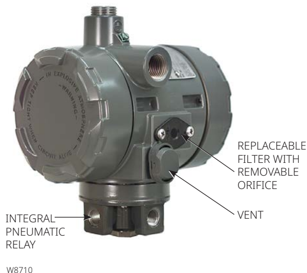
Figure 1. Fisher I2P-100 Electro-Pneumatic Transducer
