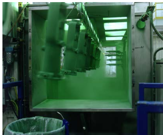
Figure 1. Powder Coating is Nearly 100% Free of VOCs
