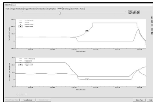
HIGH SPEED TRIGGERED DATA-STORED INSIDE THE DVC6200f DIGITAL VALVE CONTROLLER
