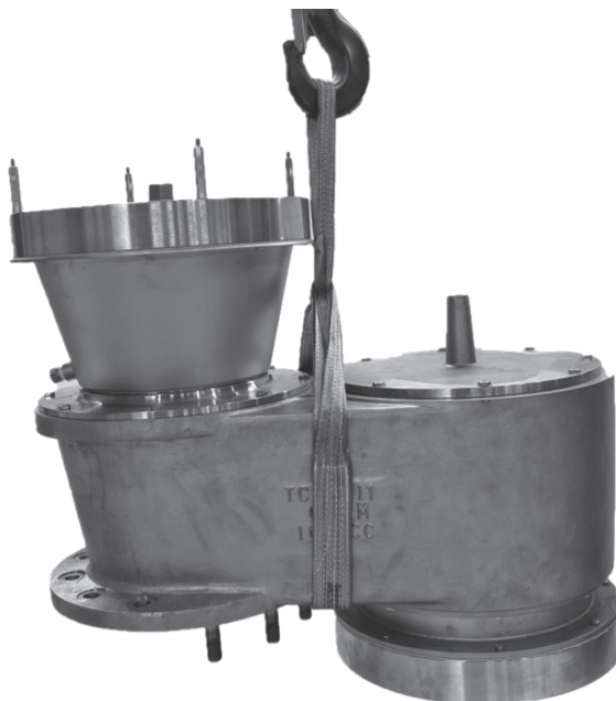
Figure 7. Hoisting for Valves
