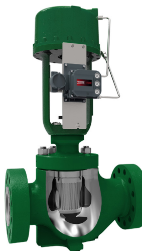
Figure 7: Dehydrator valves require 316SS bodies with 316SS or Alloy 6 trims to prevent corrosion, such as this single-seated Fisher ET or HPT (shown) valve. Valves around the CO 2 dehydrator may see noise and/or cavitation, and thus require low noise or anti-cavitation trims.
