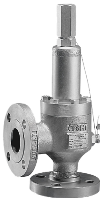
Figure 11: Proper 'snap'-acting' safety valves like this Anderson Greenwood Type 81 are preferred on CO 2 services when dry-ice formation is expected in the exhaust of the valve
