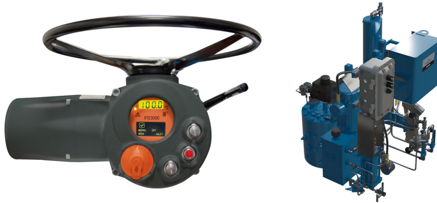
Figure 18: When air is not available, advanced electric actuators with or without spring fail assist are available (Bettis™ XTE top). For high torque applications, zero emission options, like the Shafer™ ECAT SHO (bottom), use pipeline gas pressure to drive actuator hydraulics.
