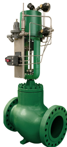
Figure 8: An anti-surge control valve, like this Fisher Optimized easy-e™ EWT, is a critical component of gas compressor operations. High-diagnostic positioners with oversized actuators and volume boosters are typically required to meet the demanding response times
