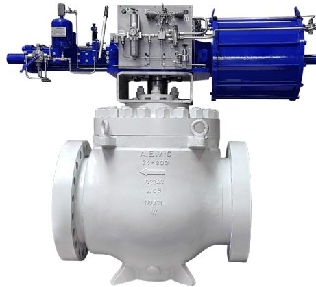
Figure 14: Double eccentric C-ball valves provide zero leakage, even in severe service applications, such as pressure swing adsorbers. The valves offer top entry and a hardened chromium carbide ball for long life. (AEV 2XC C-ball valve shown.)
