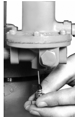
Figure 11. 161EB Series Pilot Trim Removal/Installation
