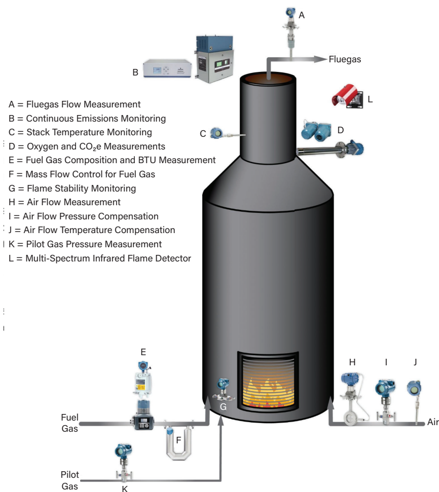
▲ Figure 5. Implementing an EMS that can analyze fired heater performance using key process measurements can help improve combustion efficiency, stability, and safety.
