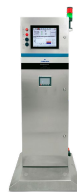
FIGURE 14 Emerson's Rosemount CT4215 Packaging Leak Detection System is able to detect minute amounts of gas leaking from a package, indicating an incomplete seal.
