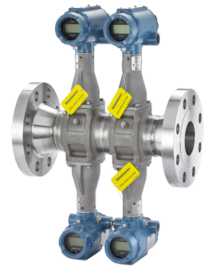
FIGURE 3 Flow meters, such as the Rosemount™ 8800 Quad Vortex Flow Meter, provide the ultimate redundant flow measurement solution to guard against spurious trips using 2oo3 voting, plus a fourth integrated transmitter for process control. The Rosemount 8800DQ040 Quad Vortex Flow Meter is rated for operating temperatures of -330°F to 842°F (-200°C to 450°C).
