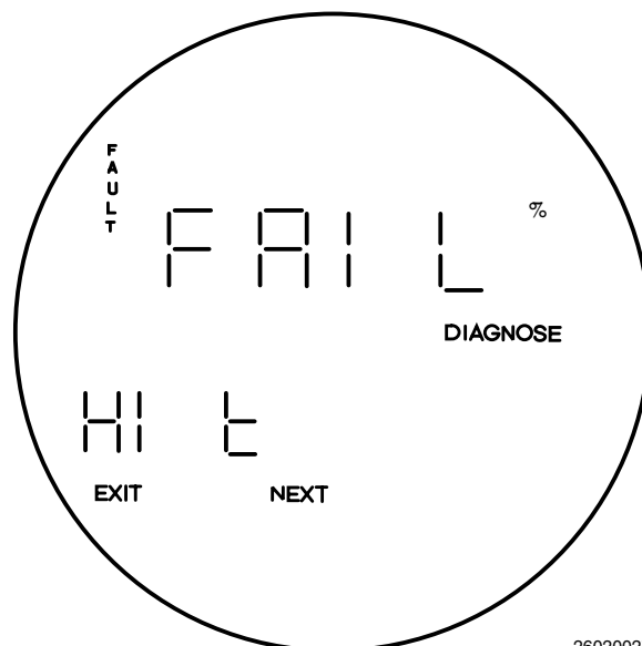
Figure 6-8. Fault 4, High Probe Temperature
