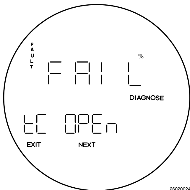
Figure 6-5. Fault 1, Open Thermocouple
