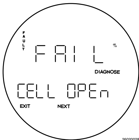
Figure 6-9. Fault 5, O 2 Cell Open
