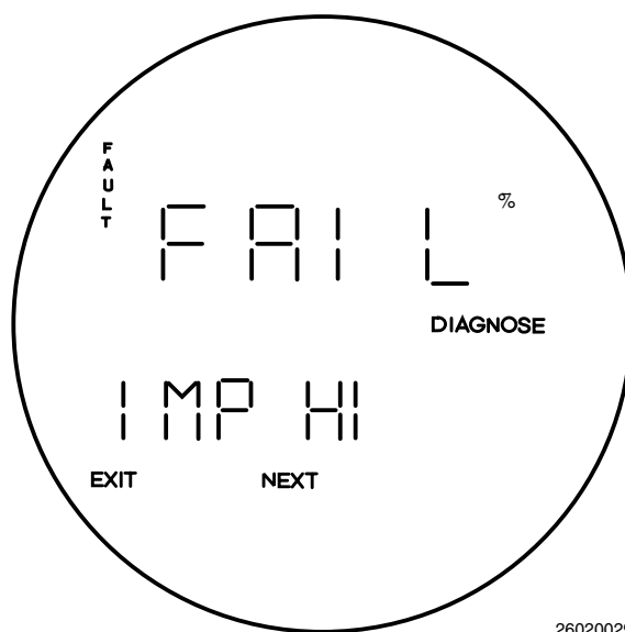
Figure 6-10. Fault 6, Cell Impedance Too High
