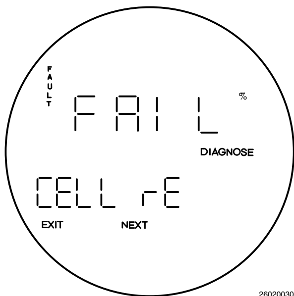
Figure 6-11. Fault 7, Reversed O 2 Cell
