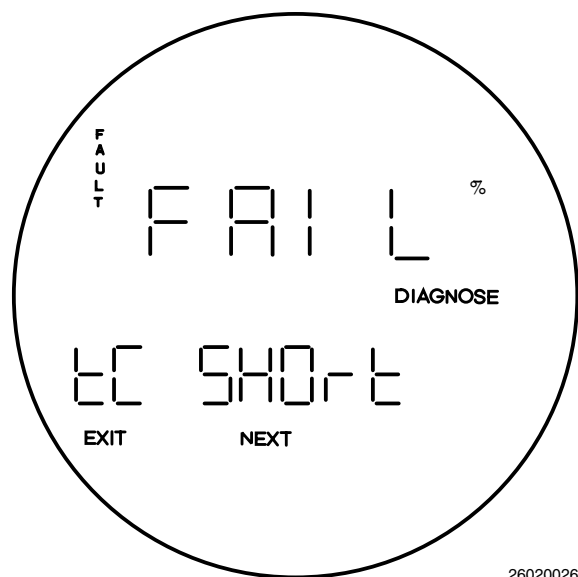
Figure 6-7. Fault 3, Shorted Thermocouple
