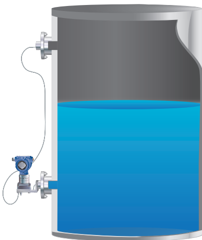
Figure 7.3.1: Illustration of a tuned system - unequal capillary length
