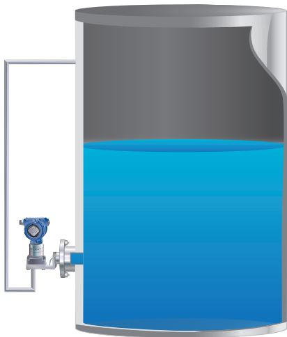
Figure 7.1.1: Illustration of a wet leg installation
