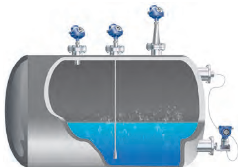
Figure 4.31.1: Sulfur solution tank level with non-contacting radar, guided wave radar and tuned system DP level
