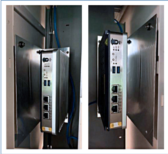
Figure 5. Vertical Mounting on Rails, Left & Right Sided.
