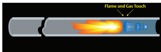
Figure 14. Concept of deflagration-to-detonation transformation in a pipe.
