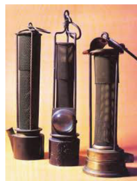
Figure 1. The earliest flame arrestors: Davy safety lamps for coal miners.
