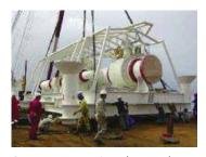
Compact rotary vane in a subsea template
